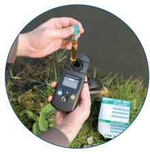
During this waiting time, the POCKET is set to zero using the blank value cuvettes supplied. All it takes is the touch of a button. The POCKET is then ready to measure the sample cuvette.
