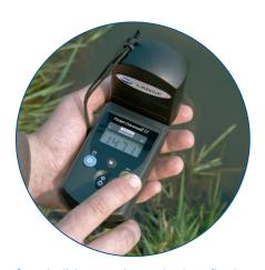
Once the light protection cap has been fitted, measurement can start: Simply press the button to read. The large display will show the result.
