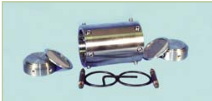
#170-45 Cell Assembly for Cement Testing, 175 mL
